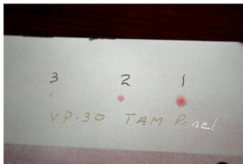
of the indications on the 50µm panel and < 75 % of those on the 30µm panel. The level 2 penetrant must show 100% on the 50µm panel and ≥ 75% on the 30µm panel.
