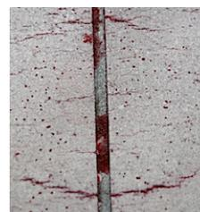
Comparison of two visible penetrant systems on a quench cracked Aluminum block
