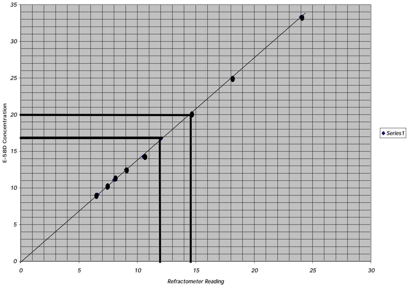
Note that these particular points do not exactly lie on a straight line. This is because of the difficulty in reading a hand held refractometer exactly. If we had used an electronic refractometer, the graph would have been more accurate. One can also derive an equation for this line, and for the line illustrated, the equation is as follows:
