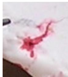
Visible penetrant indications of porosity on weld and stress cracks on metal clamp.
