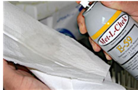
Apply **E-59** to cloth to wipe remove surface penetrant.
