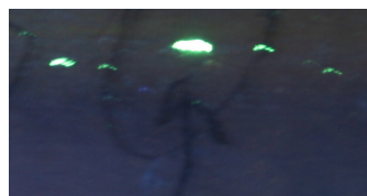
FBP-912 fluorescent penetrant indications on aluminum extrusion
