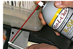
**R-504** being sprayed on cotton swab, which is used to wipe fluorescent indications. Inspector will evaluate severity of flaw indication by rate of fluorescent bleed back.
