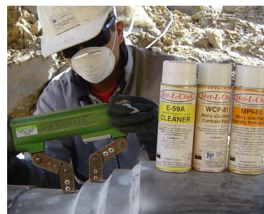
Pipe line inspection using MPI-80
